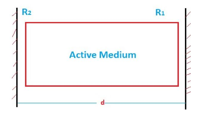
Radiation bouncing back and forth between the mirrors is amplified by the amplifying medium.
